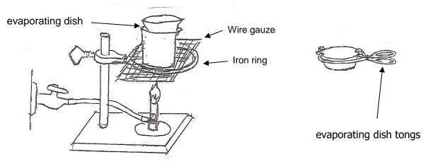
NOTE: Use the evaporating dish tongs (located in the long vertical locker at your lab bench) to handle the hot evaporating dish.
