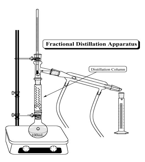
In this experiment fractional distillation will be performed in order to separate ethyl acetate from butyl acetate. Also, a comparison should be discussed with the simple distillation experiment performed previously. Assemble the apparatus as shown in the diagram. Note that its only difference from the simple distillation is the addition of the Distillation Column. To construct the column, take the air condenser and fill it up with glass beads.
