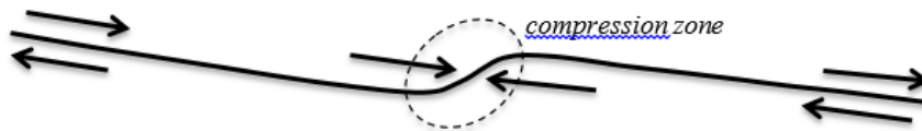
Map view of a right lateral strike-slip fault that bends, causing a zone of compression.
