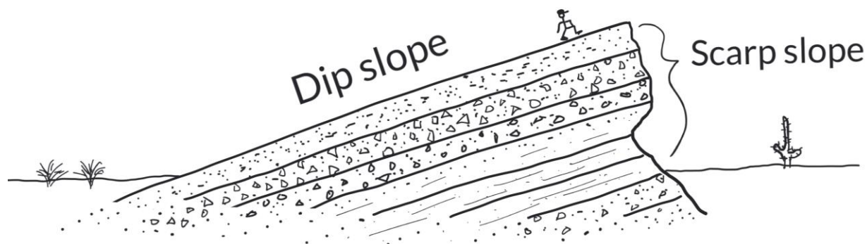
A cross-section cartoon of a cuesta, showing the dip slope and scarp slope.
