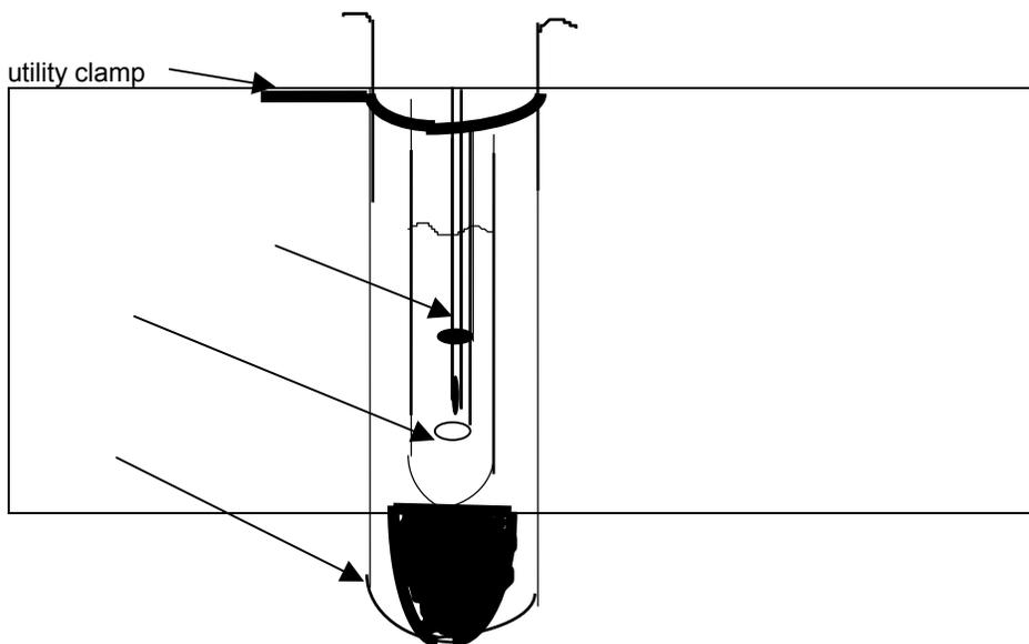
6. After you have obtained the freezing point data, remove the assembled test tubes from the ice bath, cork the test tube containing cyclohexane, and allow warming up to about room temperature.
