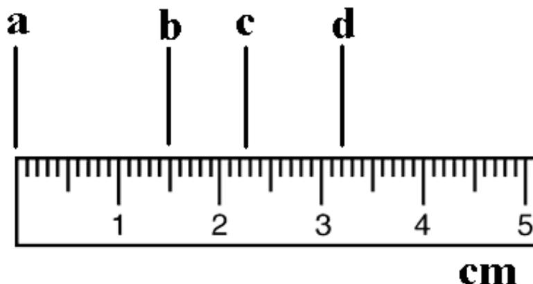
The lines on this ruler are to the 1/10 or 0.1 cm. So the measurement must include one estimated digit which would be to 0.01 cm or 1/100 cm. In the case of measurement "a" the student would write 0.00 cm. The marks on the ruler with numbers are cm and the smallest marks are mm. The measurement would be written with the units "cm" and the number must go to 0.01 cm. If the measurement falls directly on the line the last digit would be "0". In measurement b the value is 1.50 cm not 1.5 cm. If the
