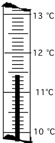
The mercury in this thermometer is between 11.4 and 11.5 you need to estimate (interpolate) the last digit. The reading should be written as 11.42 °C . (It is understood that it is 11.42 °C  $\pm$  0.01°C.)
