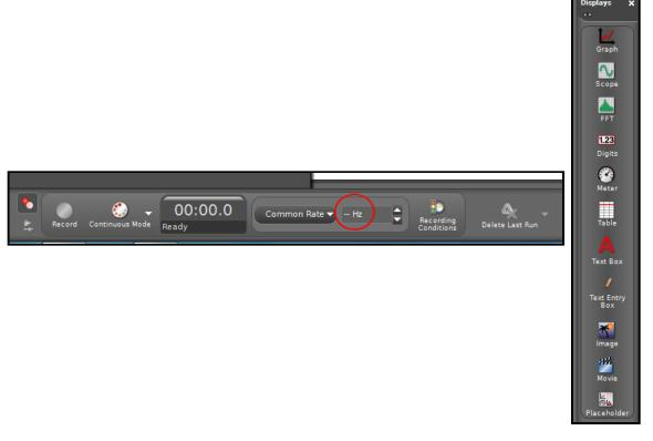
The control in the red circle above is important: it allows you to set how often the interface samples the sensor. (More on that in other labs). The experiment is started with the record button, but start and stop conditions can be applied:
