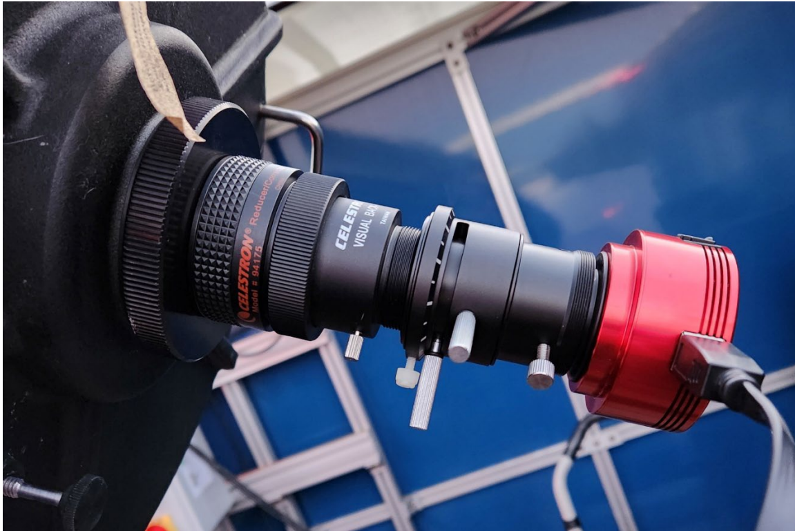
Figure 11 - This is what the stack of equipment looks like for taking wider field planetary and lunar images. The 0.63x reducer lens mounts to the back of the C14 first, followed by the 2" to 1.25" adapter, the ADC, and finally the camera.
