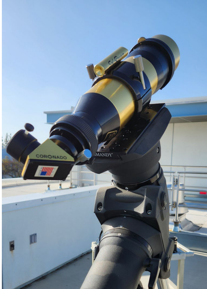
Figure 2 - Coronado H-alpha solar telescope in place on the CGEM DX mount
