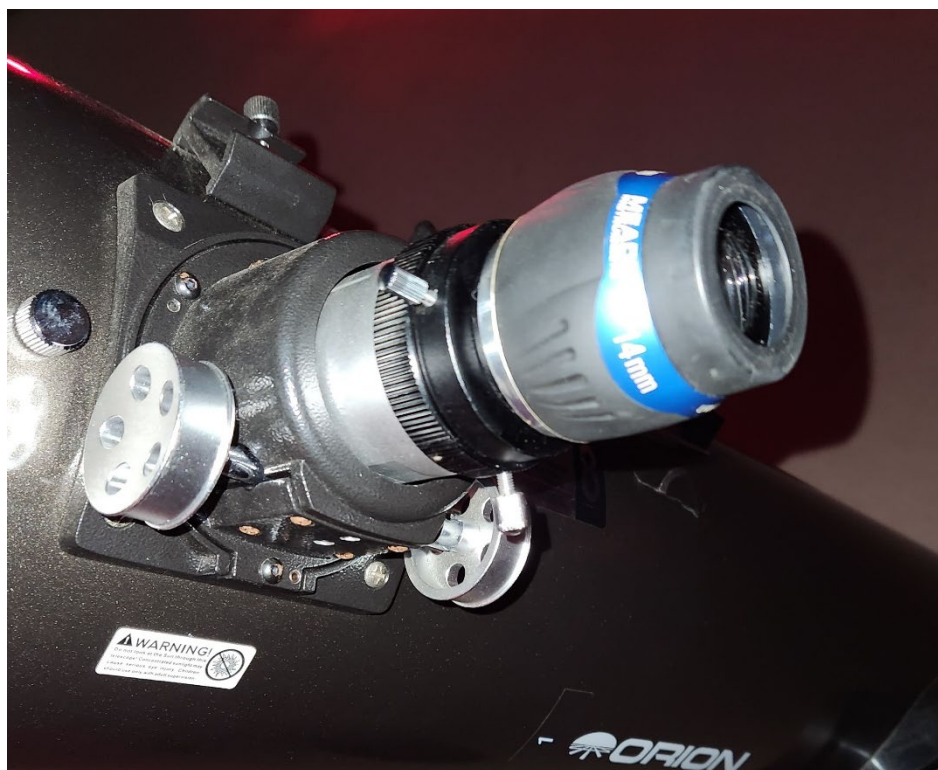
Figure 8 - Focuser with the 1.25" adapter and a 1.25" diameter eyepiece in place. This is the most common configuration that students will use.
