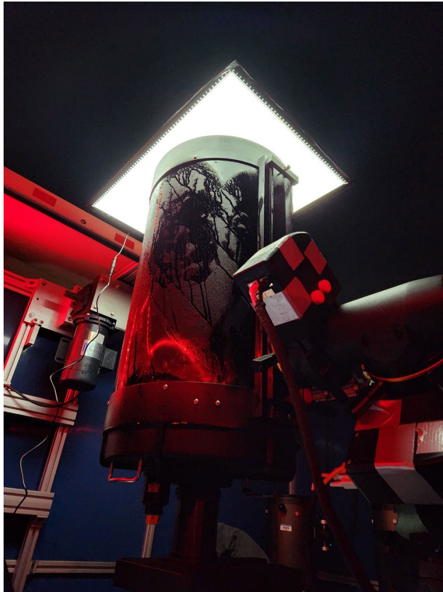
Figure 32 - Setup for taking flat frames with the C14; the light panel that is on top of the telescope can be found in the bottom of the cabinet in the observatory
