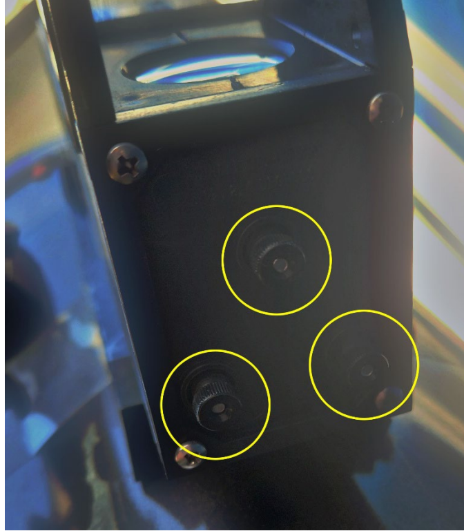
Figure 5 - Use these three screws to adjust the position of the bullseye when viewing through the Telrad
