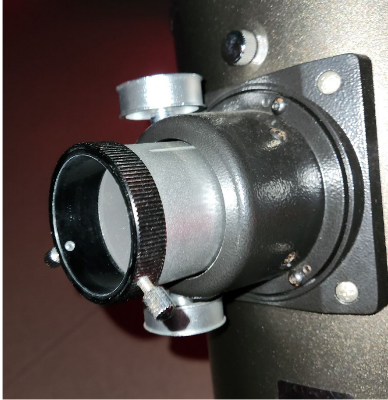
Figure 6 - Focuser on an 8" Dobsonian with no adapter and no eyepiece present
