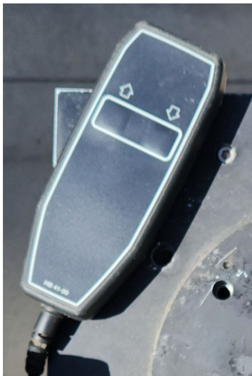
Figure 10 - Hand control for raising and lowering the telescope pier
