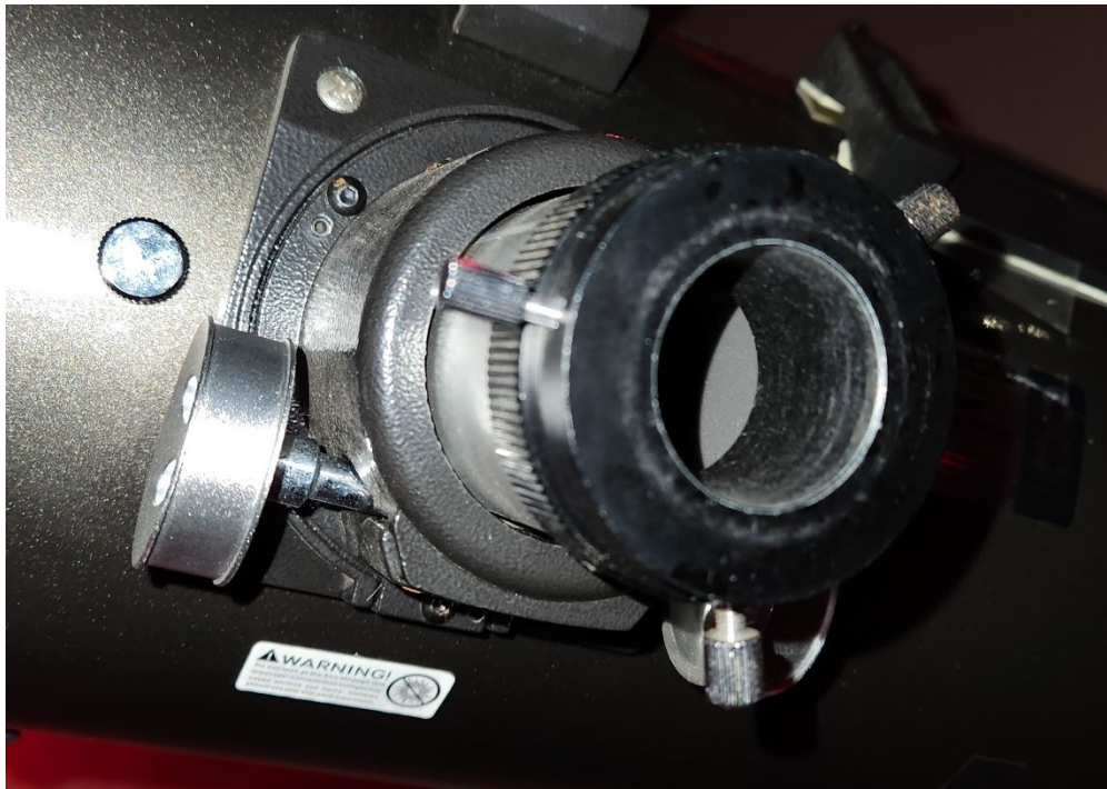
Figure 7 - Focuser on an 8" Dobsonian with the 1.25" adapter in place, but no eyepiece
