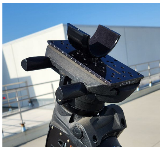
Figure 1 - Losmandy plate with bracket for mounting a Coronado solar telescope on the CGEM DX equatorial mount
