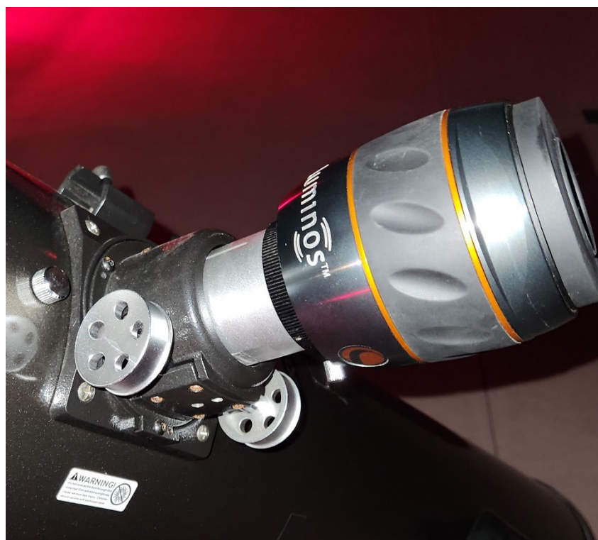
Figure 9 - An option for giving students a very wide-field view is to use one of the 2" diameter eyepieces from the top shelf of the cabinet in the observatory. Remove the adapter collar before inserting one of these eyepieces.
