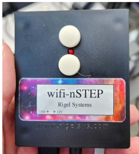
Figure 65 - The controller for the focuser for the 14-inch SCT
