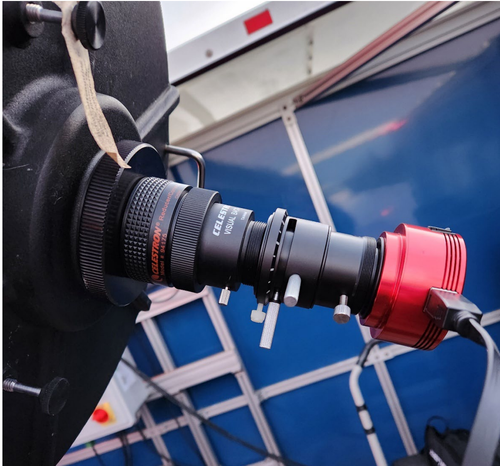
Figure 69 - This is the setup for wider field planetary imaging. The 0.63x reducer attaches to the back of the telescope first, followed by the 2" to 1.25" adapter, the ADC, and the ZWO ASI224MC camera.
