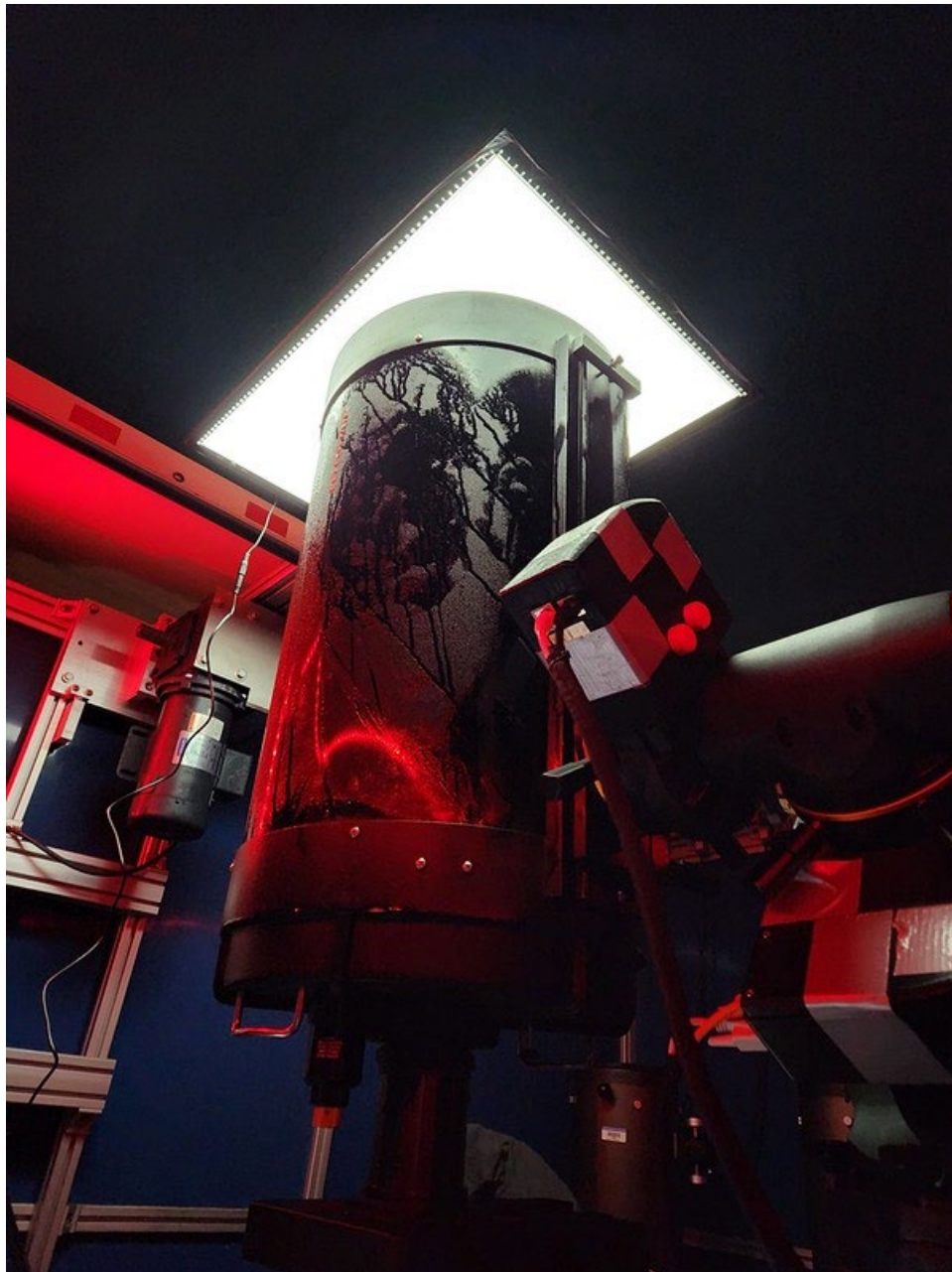
Figure 15 - This is the setup for taking flat frames with the 14" telescope on campus.
